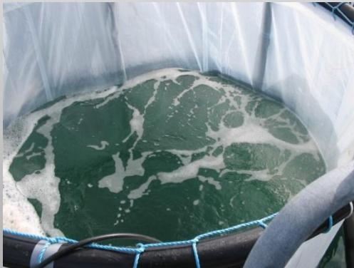
**HOWTO: aeration of the mesocosms ( $\sim 30\text{m}^3$  each) with air enriched with CO<sub>2</sub> at target levels**
