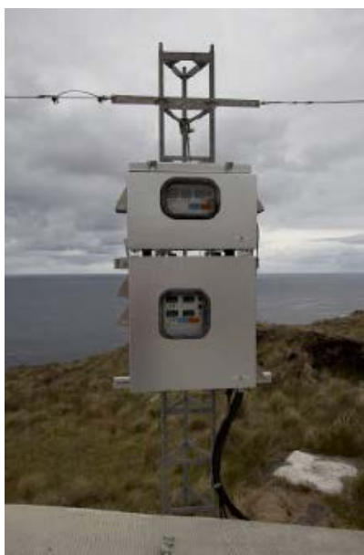
Figure 5. Tekran front-end modules 1130 and 1135 installed on the roof Pointe Benedicte's laboratory at Amsterdam Island ( 37,79604^{\circ}\text{S} , 77.55095^{\circ}\text{E} ). (from Barret M., A. Dommergue, C.P.)
