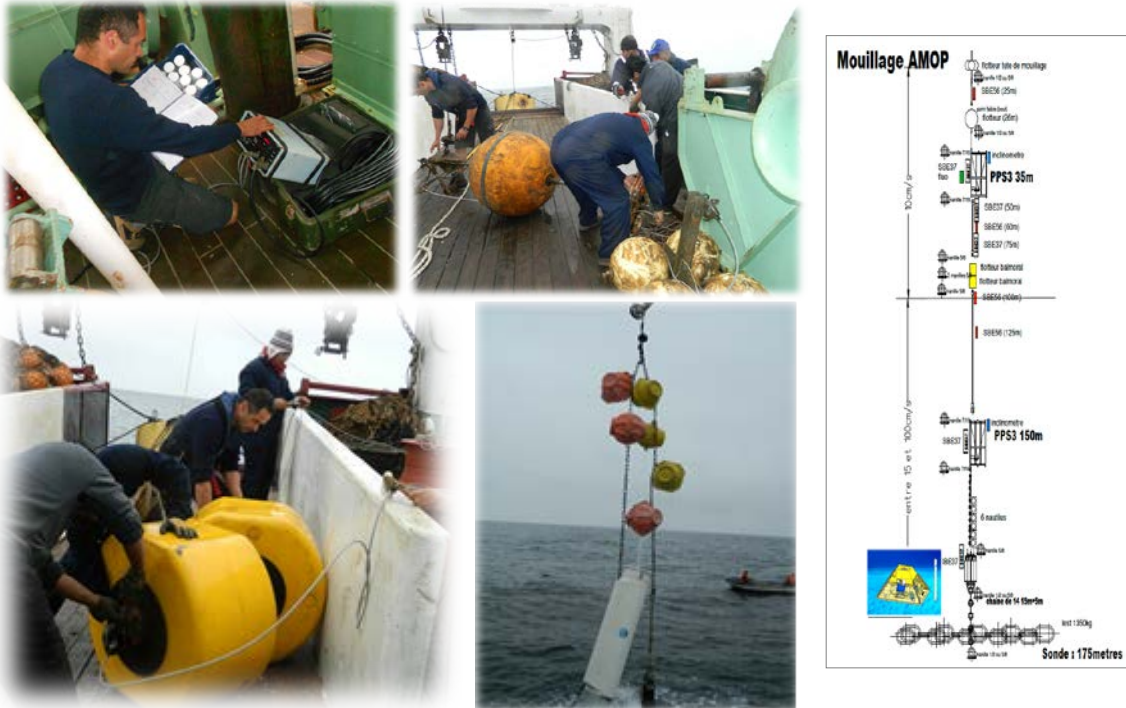
Recover and deployment of the subsurface AMOP mooring- R/V Olaya, June 2013 courtesy IMARPE Peru
