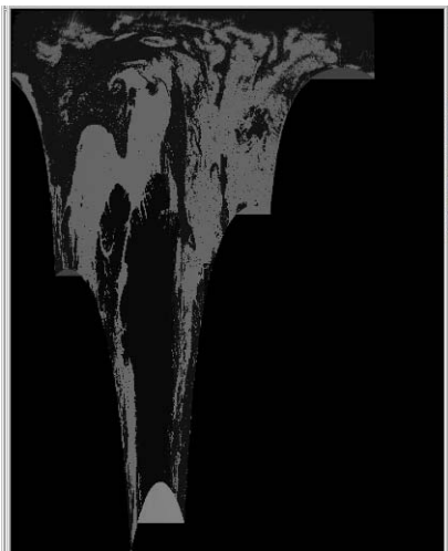
A raw, uncolored Level 2 swath image of sea ice properties from MODIS. After conversion to a regular grid (below) with HEG, the data fit neatly onto a GIS base map (in MapWindow)
