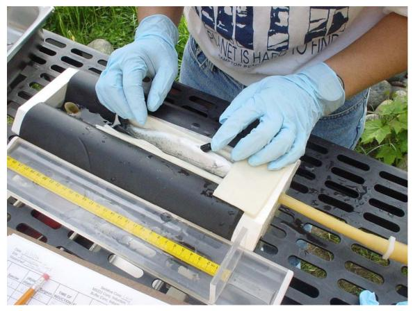
A scientist implants a tag into an anaesthetized steelhead trout smolt as part of the Pacific Ocean Shelf Tracking project.
